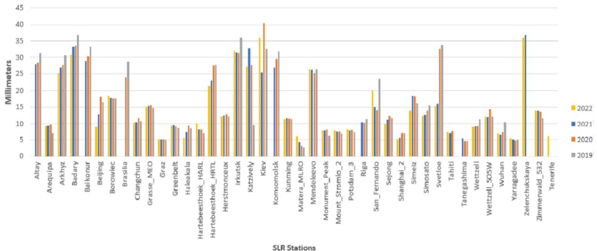
Figure 2-10. LAGEOS range precisions measured by ILRS network stations
